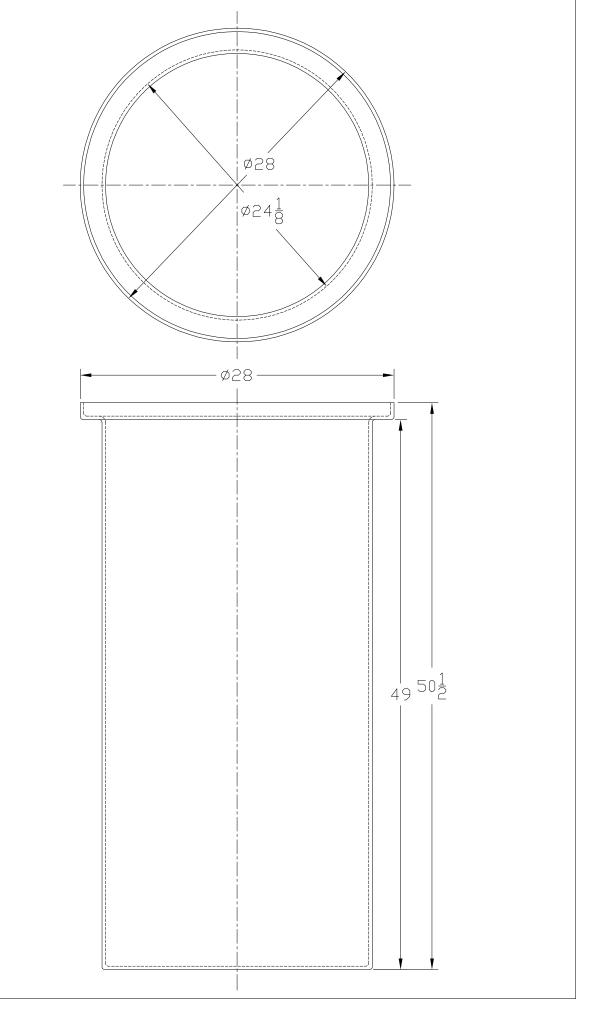
ALL DIMENSIONS SHOWN ARE OUTSIDE PART DIMENSIONS IN INCHES, AND VARY BY THE STANDARD ROTATIONAL MOLDING TOLERANCE OF +2;-3%.
