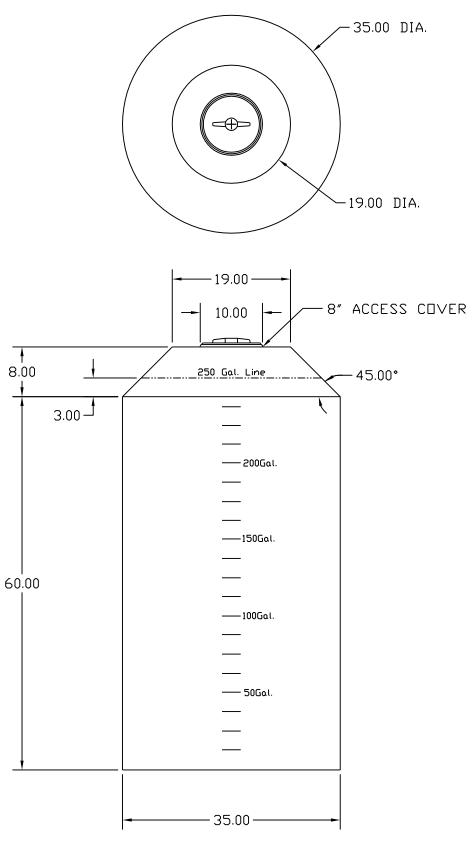
ALL DIMENSIONS SHOWN ARE OUTSIDE PART DIMENSIONS IN INCHES,AND VARY BY THE STANDARD ROTATIONAL MOLDING TOLERANCE OF 2% TO 3%.
