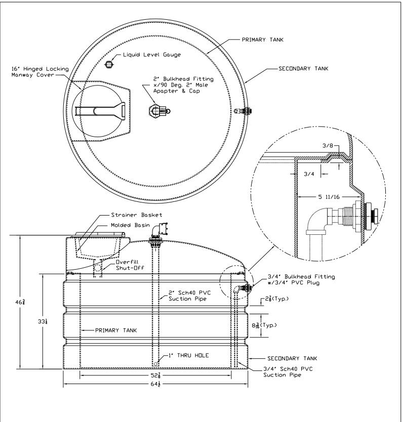
ALL DIMENSIONS SHOWN ARE OUTSIDE PART DIMENSIONS IN INCHES,AND VARY BY THE STANDARD ROTATIONAL MOLDING TOLERANCE OF 2% TO 3%.
