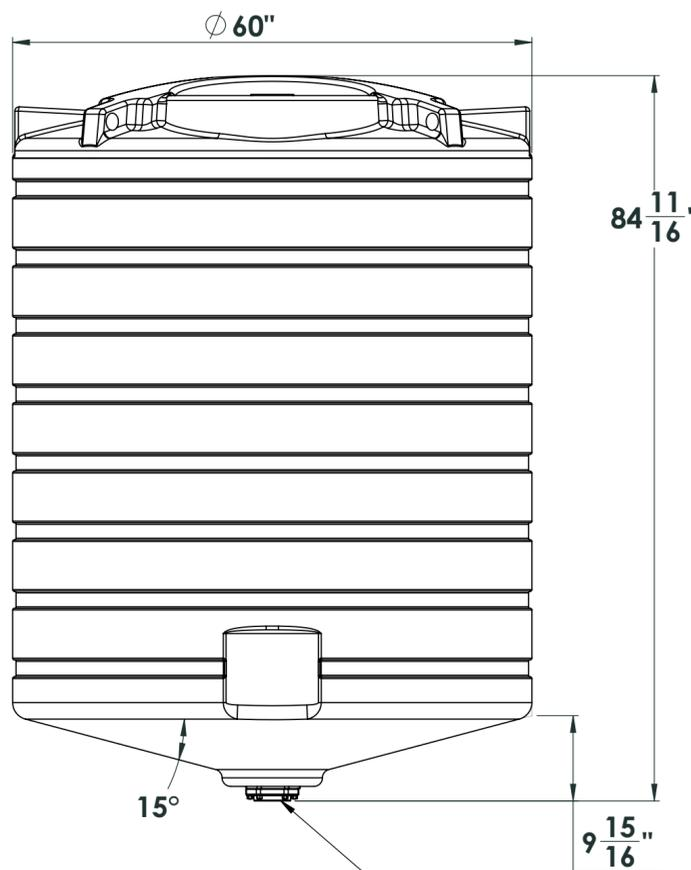
3 inch bolted - bottom drain fitting
