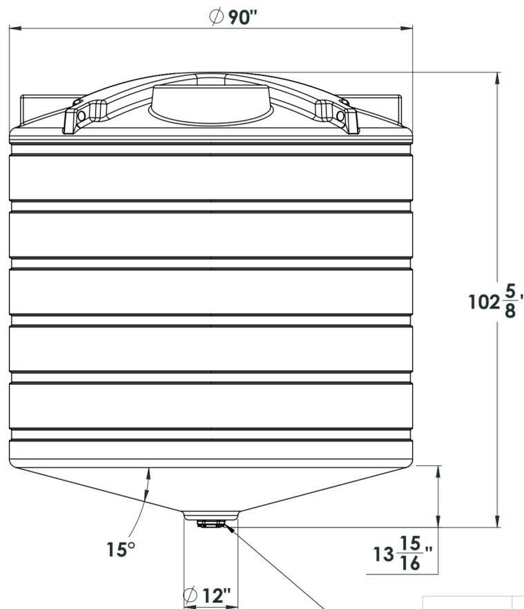
3 inch bolted - bottom drain fitting
